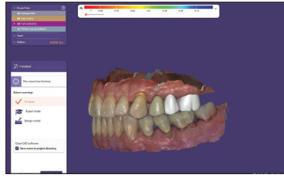
Figure 4. The margins and contours were adjusted with "free form" in Wizard Mode.
